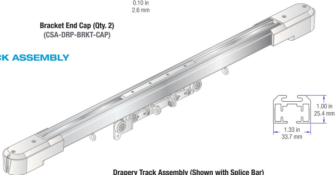
**Drapery Track Assembly (Shown with Splice Bar)**
