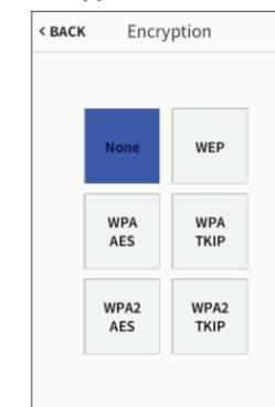
8. Tap the appropriate type of encryption used by the access point, and then tap **< BACK**.
