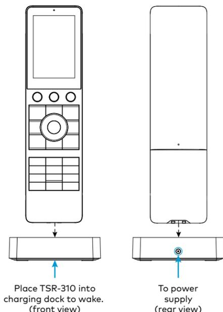
**NOTE:** Prior to operation, allow the remote to remain in its charging dock for up to three hours until fully charged.
