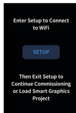
Tap **SETUP** to enter the built-in setup screens. The TSR-310 main setup screen is displayed.
