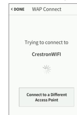
If the connection to the access point is successful, the WAP Connect screen indicates that the connection is active.
