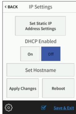
2. Tap **On** or **Off** under **DHCP Enabled** to enable or disable using DHCP (dynamic host configuration protocol).
