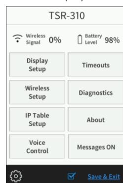
Configure device settings for the TSR-310 using the built-in setup screens or using the web configuration interface. For more information on configuring the device, refer to the TSR-310 Supplemental Guide (Doc. 8226) at [www.crestron.com/manuals](http://www.crestron.com/manuals).
