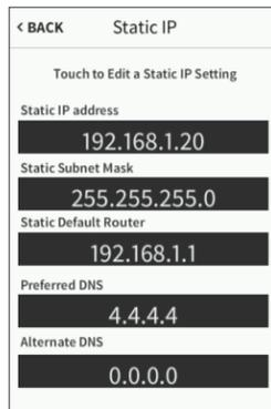
4. Tap the fields under **Static IP Address**, **Static Subnet Mask**, **Static Default Router**, **Preferred DNS**, and **Alternate DNS** to enter the required information using the on-screen keypad.
