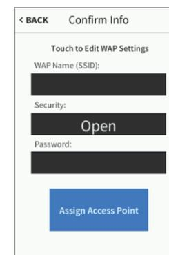
5. Tap the **WAP Name (SSID)** field on the **Confirm Info** screen, and enter the name of the access point using the on-screen keyboard.
