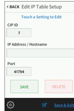
3. Tap the text field below **CIP ID** to enter the appropriate CIP ID using the on-screen keypad.
