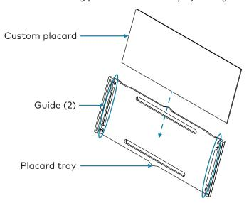
4. Reinsert the tray into its slot in the DSS-100 until it snaps into place.
