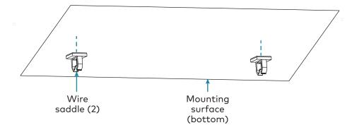
6. Route the USB-C<sup>™</sup> connector end of the provided USB cable from the power source to the DSS-100 mounting location through the wire saddles. Each wire saddle provides a clip that can be opened to insert the cable.
