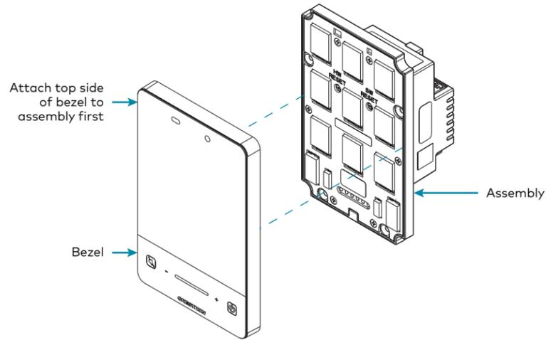
**NOTE:** If the bezel is removed and then reattached to the assembly, there is a 20-second delay before the buttons are functional.
