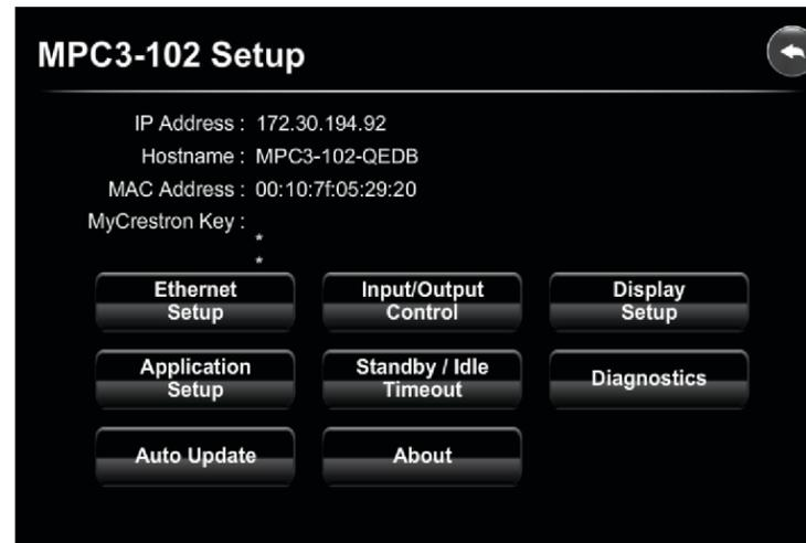
The Setup page displays the IP address, hostname, and MAC address of the MPC3 device, as well as a key that is used to register the MPC3 device with the MyCrestron service.
