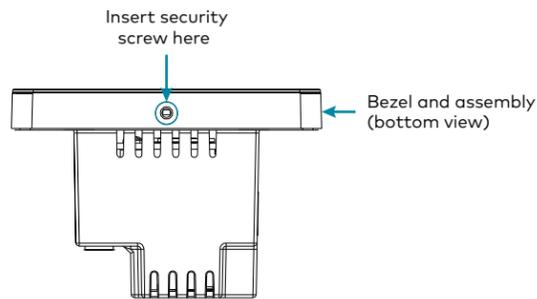
**NOTE:** To remove the bezel from the assembly (required to access the icon chips and the reset buttons), unscrew the security screw from the bottom of the bezel (if installed), and then gently pull the bezel, bottom side first, away from the assembly until the magnetic hold is broken.
