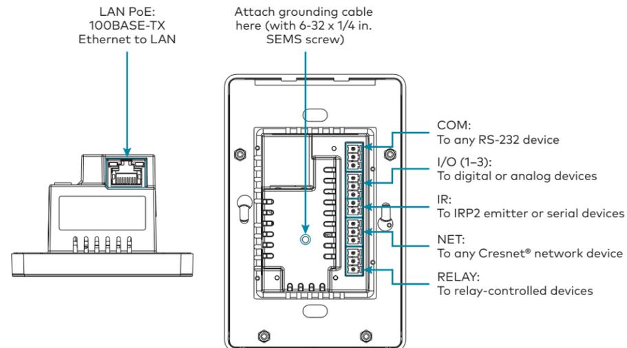
Observe the following when making connections to the MPC3 device:
