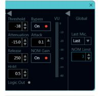
Controls and parameters common with the Gate object Controls and parameters unique to the AMIX object are highlighted. This includes global parameters that affect all AMIX objects in the DSP
