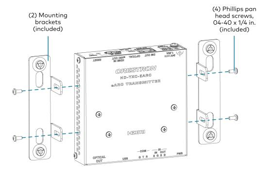
2. Position one of the mounting brackets so that the holes align with the holes in the rack rail.
