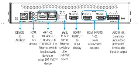
**NOTE:** The DM-NVX-350 and DM-NVX-351 can be configured to use either the DEVICE port or the HOST port. Both ports cannot be used simultaneously.
