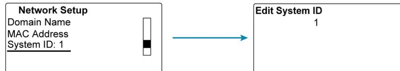
3. Select a unique system ID for the DM switcher. The recommended setting ranges from 2 to 64.
