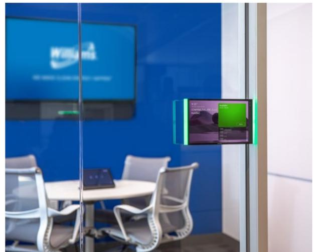
XiO Cloud allows the Williams IT team at HQ to monitor devices, update software, and easily view the status of the devices in their rooms. It also proactively notifies IT when a device is down rather than only being alerted when an employee encounters a faulty room. For the Oklahoma-based IT team, they are now able to remotely assist an employee at any office location by controlling their touch screen to get a meeting started or help with any of the device features.
