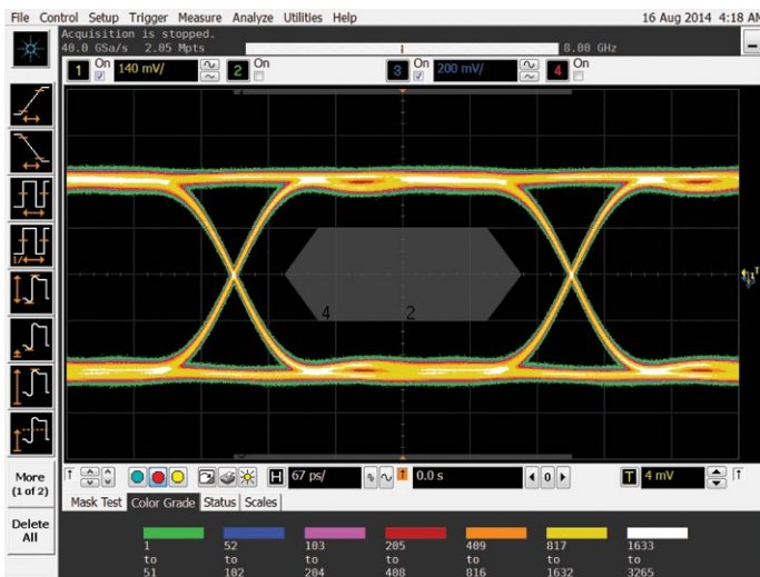
This shows a clean 4K eye diagram; The eye is wide open because the system under test has more than enough bandwidth to support 4K.
