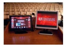
This level of production will require an expert at the controls, so Griffes installed a 15in. Crestron V15 V-Panel touchscreen in the equipment area for the technical operator to use. He also designed the system to work on a day-to-day level without a technician. "We put a second 15in. V-Panel in the main podium so that the presenter can control everything," he says. Griffes
