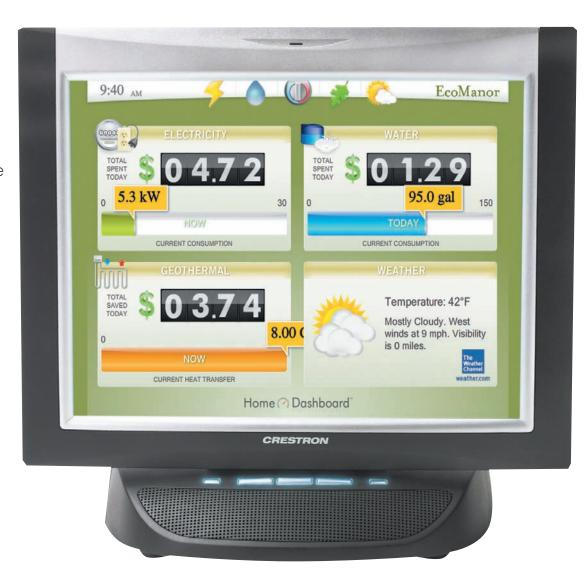
The environmental control dashboard displays real-time data on utility consumption throughout the home in terms the home owner can understand. It's displayed here on Crestron's TPMC-15 touch screen, however it can be accessed from anywhere. See the live demo at: http://www.crestron.com/features/go\_green/
