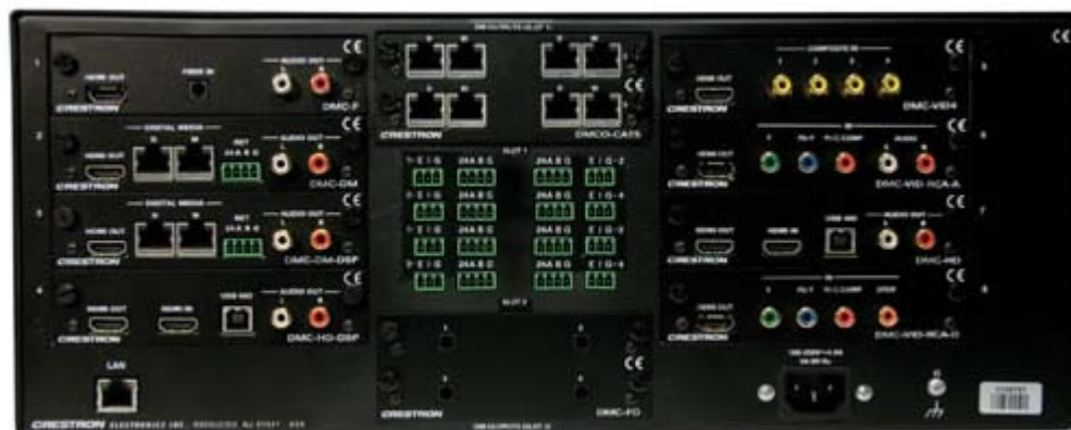
The rear of the DM-MD8X8 switcher showing a selection of input and output modules.
