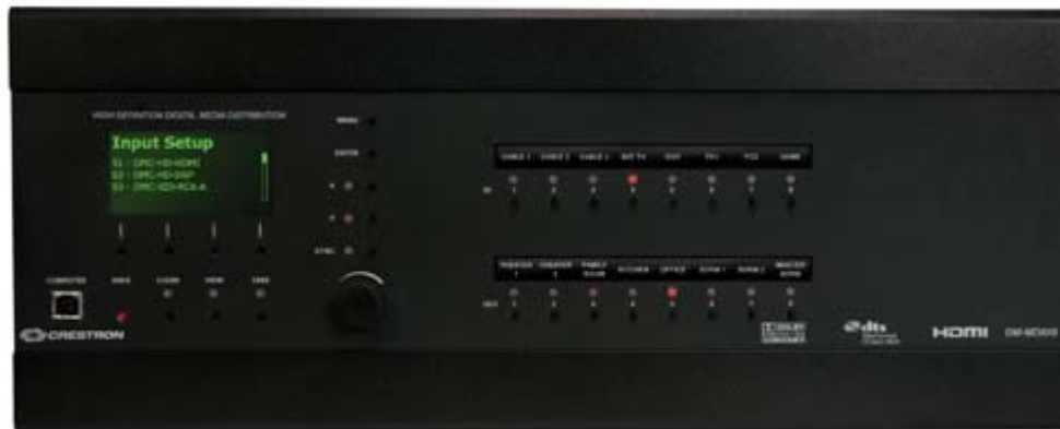
The DM switcher, shown here in an 8x8 version, serves as the central hub of the DigitalMedia system.
